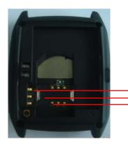
Line up the 3 connectors on battery with these 3 connections.
